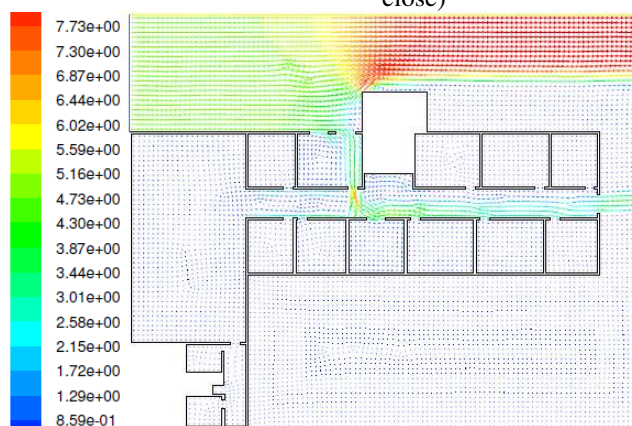
Fig. 10 Velocity vectors around the school (aisle window: open)
