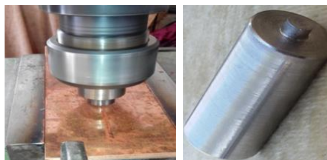
Fig. 2 The tool used and its interaction with the part in the friction stir processing.
