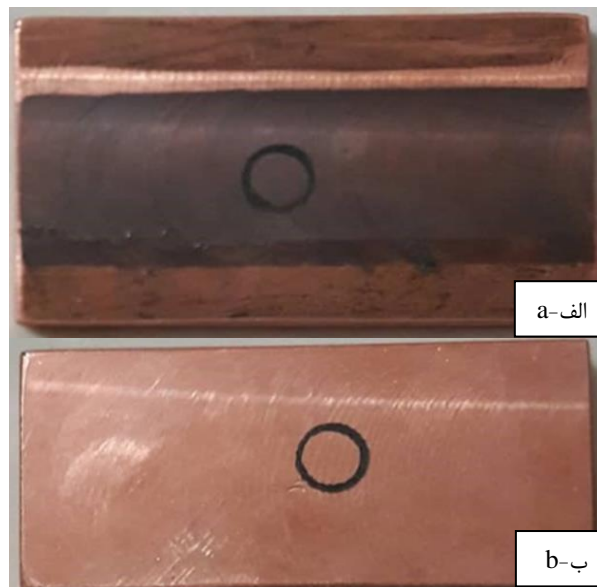
Fig. 7 Wear Test samples marked with numbers 01 and 08 Copper Specimen with and without FSP.
