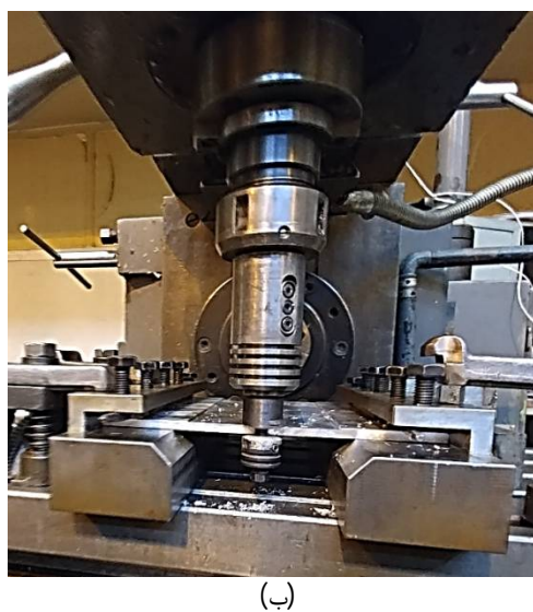
Fig. 1 The image of the floating bobbin tool and its fixture; a. schematic image and b. the real picture
