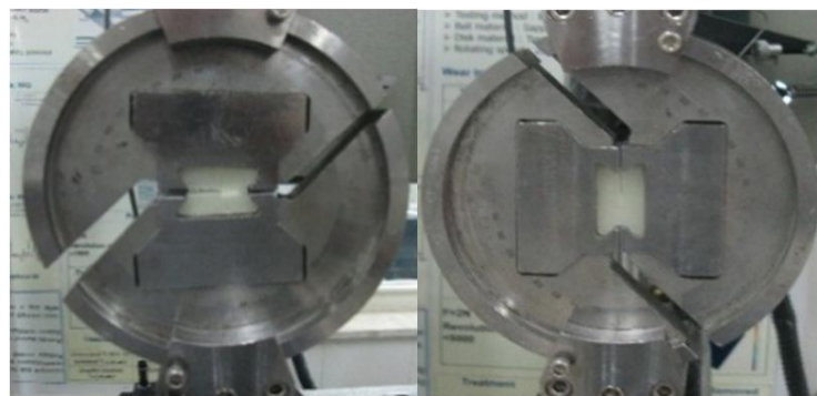
Fig. 7 Butterfly specimen test in mode-I & mode-II with new loading fixture
