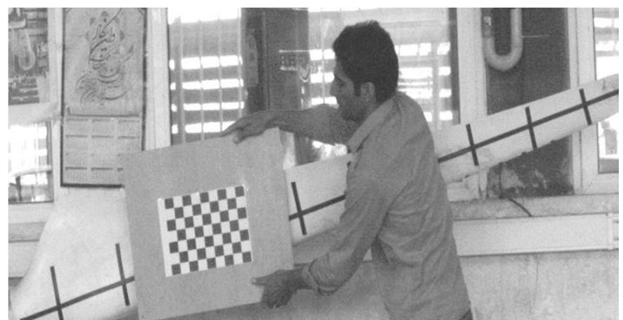
Fig. 7 Targeted plane placed on the wind turbine blade body
