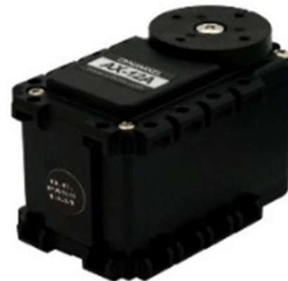
(f) Dynamixel AX-12 motor used in robot
