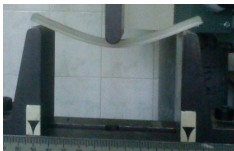
Fig. 2 Configuration of three-point bending test
