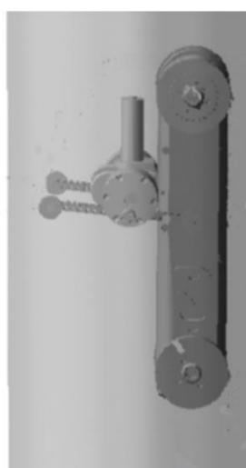
Fig. 15 Module functionality in robot movement in high inclination pipes
