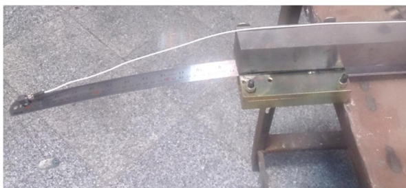
Fig. 8 Test set-up (beam with initial displacement)
