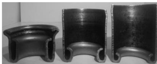
Fig. 18 Internally inverted sectioned tubes for the impact velocity of 89 m/s, (respectively from right to left, m=175, 264 & 475 gr)
