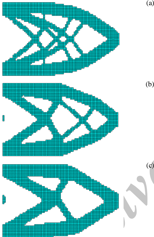
Fig.4 Optimal topology for cantilever beam with ER = 1\% : (a) r_{min} = 1.5 \text{ mm} ; (b) r_{min} = 2 \text{ mm} ; (c) r_{min} = 3 \text{ mm}
