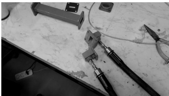
Fig. 9 A view of Short Load calibration step
