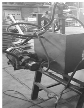
Fig. 4 Hydraulic power supply unit used in experiments (power pack).
