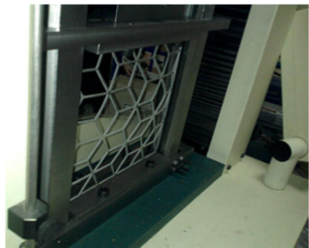
Fig. 24 Global buckling mode for diacube-B model in experiment
