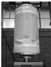
Fig. 7 Cylinder after buckling
