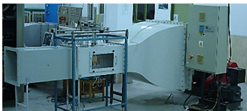
Fig. 2 view of open circuit wind tunnel
