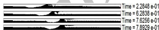
Fig. 3 Mesh independence of slug regime in channel flow with k-ε RNG turbulent model
