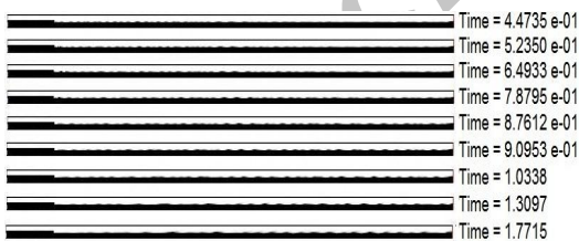
Fig. 7 slug modeling with Standard k-ε turbulent model at 12 m/s velocity difference
