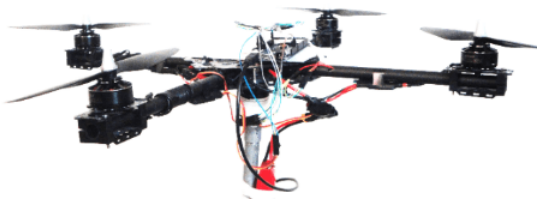
Fig. 10 Quadrotor on the experiment base with three degree of freedom
