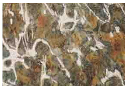
Fig. 2 GSH48 graphite steel by pearlitic and dispersed carbide(x200)
