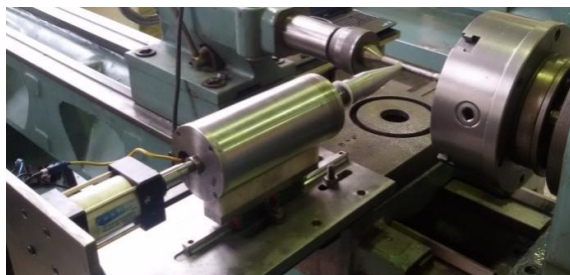
Fig. 10 Assembling of UPT equipment on the lathe
