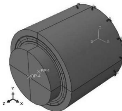
Fig. 10 Applied constraints for modelling of the extraction strength
