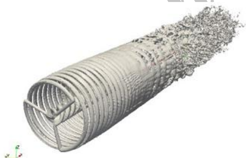
Fig. 17 Vortex isosurface contours and wakes structure
