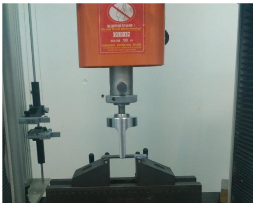
Fig. 1 Three point bending test setup, mounted on a computer controlled universal compression testing machine.
