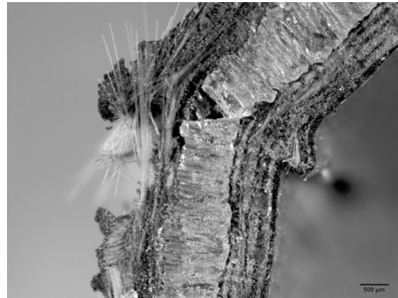
Fig. 5 Optical microscope image of the failed FMLs in the three point bending test
