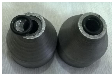
Fig. 11 Arrangement of O-ring on the conical piece
