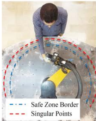
Fig. 7 The operator is forcing the sensor which is installed in the robot end-effector
