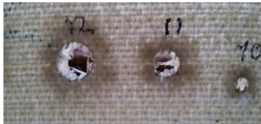
Fig. 6 Matrix fracture and uncut fiber in the hole
