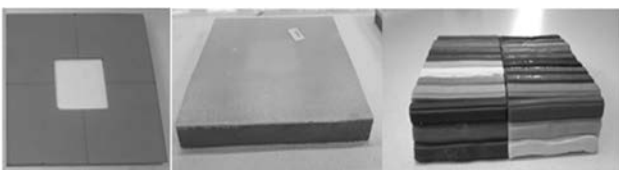
Fig.4 Ceramic/composite target, front view (left), back surface (center) and backing colored clay block (right)
