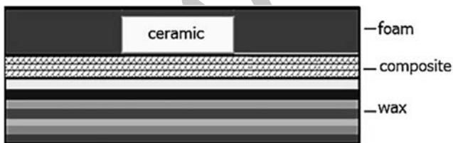
Fig. 3 Schematic of Ceramic/composite sample and arrangement of layering.
