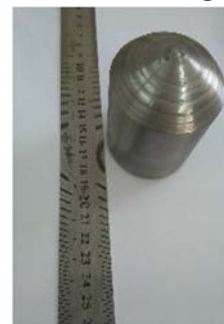
Fig. 10 Head of hammer for generating point load
