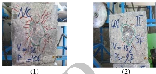
Fig. 18 Concrete after impact with gas gun (1) Normal concrete (2) Rubberized concrete contained 40% rubber and silica fume
