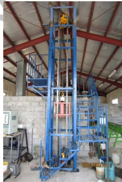
Fig. 9 Drop hammer device
