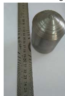
Fig. 10 Head of hammer for generating point load
