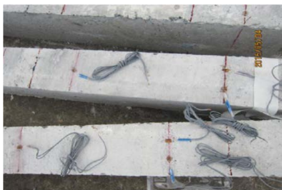
Fig. 11 Strain gages attached to rubberized concrete
