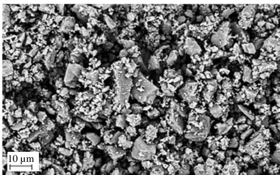
Fig. 3 SEM micrograph of (a) SiC particles and (b) CaCO 3 powder
