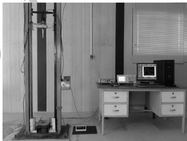
Fig. 6 A picture of the drop-weight impact testing machine and the data acquisition system (the experimental set up)
