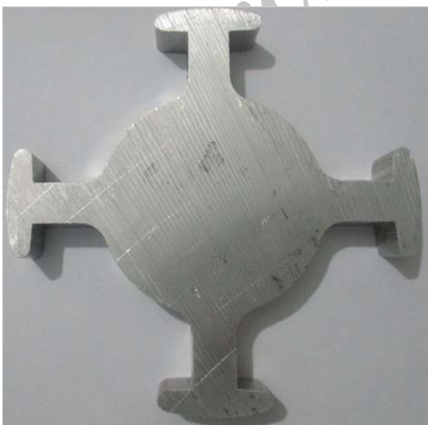
Fig. 11 A view of the section created in part by using first die
