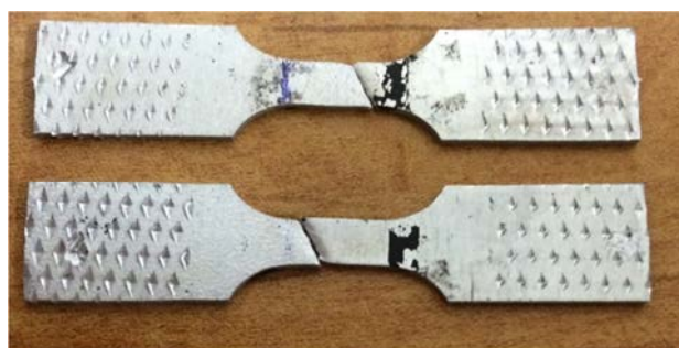
Fig. 2 fracture of sample after uniaxial tensile test
