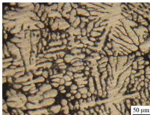
Fig. 5 The optical micrographs of As cast A356 alloy
