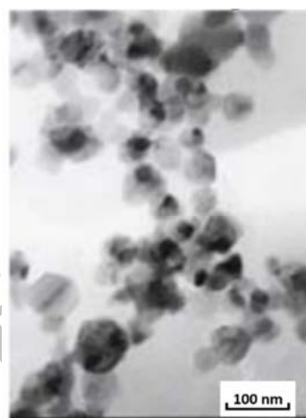
Fig. 2 TEM micrographs of As-received SiC nano particles
