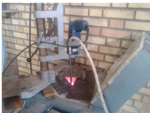
Fig. 4 The stir casting system used in this study
