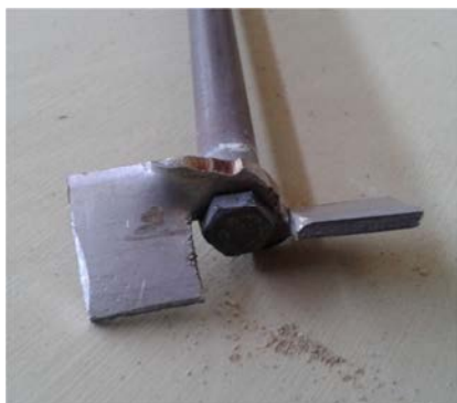
Fig. 3 View of stainless steel stirrer
