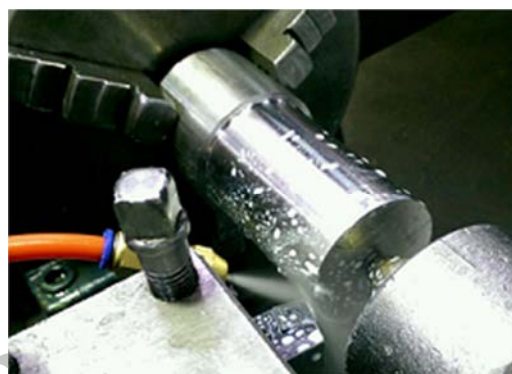
Fig. 2 Nozzle MQL, tool and workpiece setup
