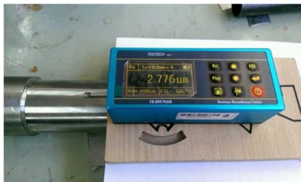
Fig. 1 Image Roughness tester and Workpiece
