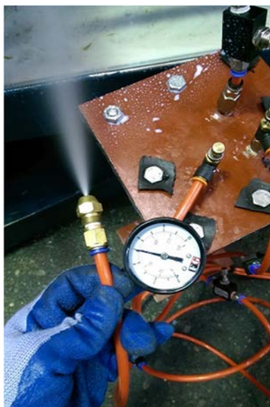
Fig. 3 A view of the spray produced in the MQL device
