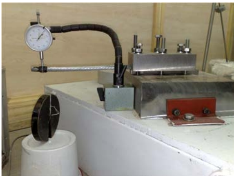
Fig. 5 Bending test to estimate the EI of messenger cable
