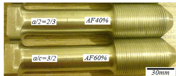
Fig. 5 Two samples of cracked specimens with \xi = 0.4
