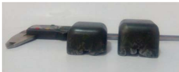
Fig. 13 Samples produced by hydro mechanical deep drawing with drawing ratios of 1.8 and 2.2
