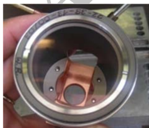
Fig. 3 The optic system protector installed in the tip of laser gun
