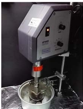
Fig. 2 Using of probe sonicator and ice bath
