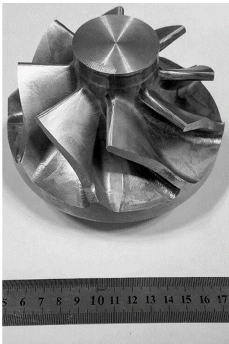
Fig. 20 machined impeller by 3+2-axis machining method
