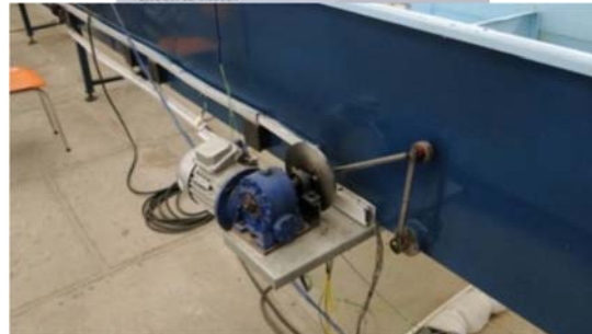
Fig.5 paddle-type wave-maker system
