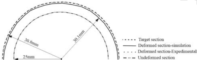
Fig. 11 Comparison of target profile with simulation and experimental profile for bulged sample
