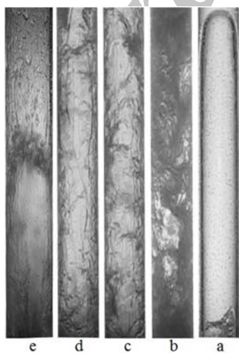
Fig. 3 Flow patterns in tube with inner diameter of 60 mm a) slug, b) churn, c) churn-annular, d) annular, e) reverse flow
