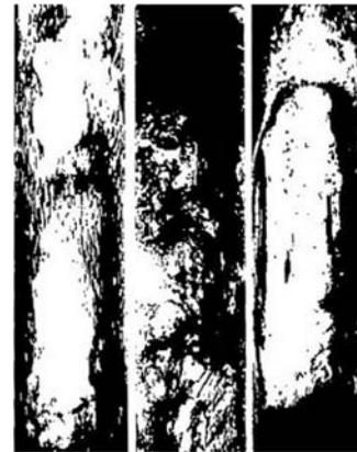
Fig. 10 Binary Images of Flow patterns in tube with inner diameter of 110 mm
