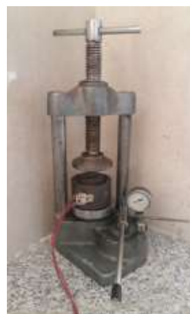
Fig. 5 Press for micro extrusion and die setup.
