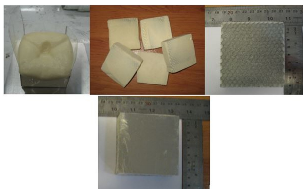
Fig. 3 Preparation of sandwich panels filled with foam
