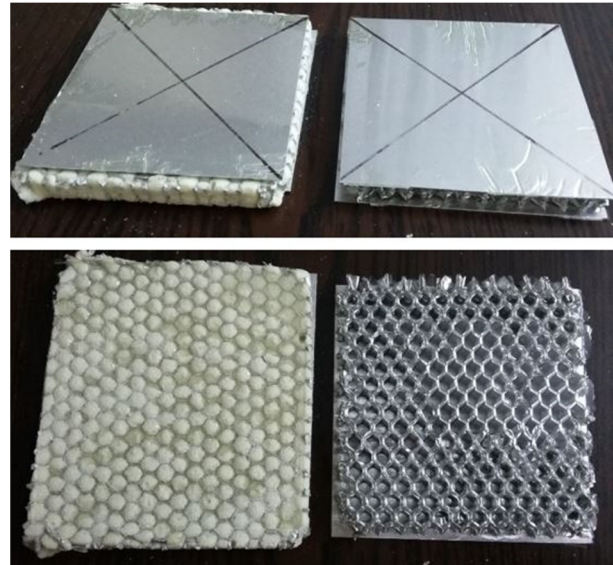
Fig. 6 empty and foam filled sandwich panel under distributed loading (from top to bottom, sandwich structures and sandwich panels without face sheet)
