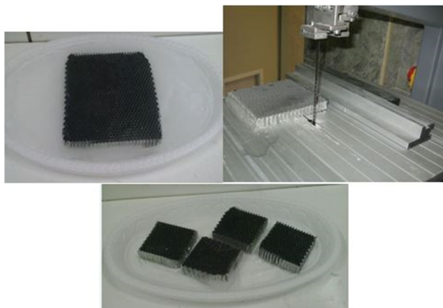
Fig.2 Preparation and cutting of honeycomb structures
