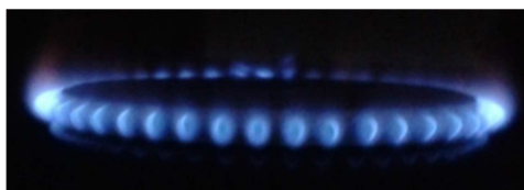
Fig. 7 Conventional burner flame
