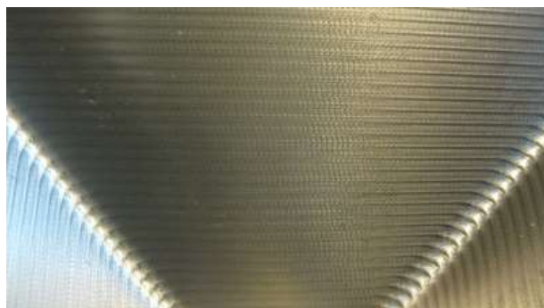
Fig. 25 Surface roughness of formed part at tool rotation speed of 5000 RPM
