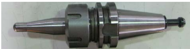
Fig. 7 hemispherical head tool with 9 mm diameter
