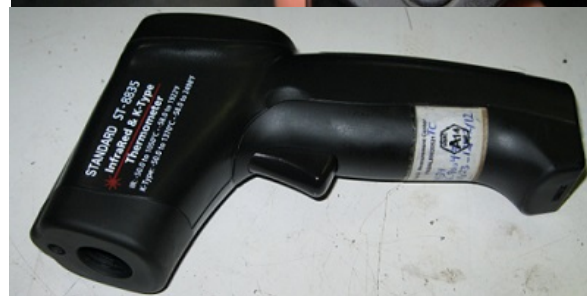
Fig. 11 Infrared thermometer to measure forming location temperature
