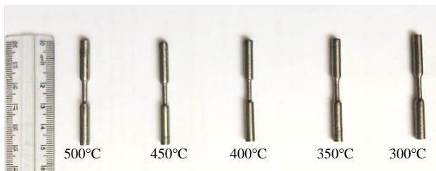
Fig. 4 Prepared samples for tension test from extruded specimens at certain temperatures
