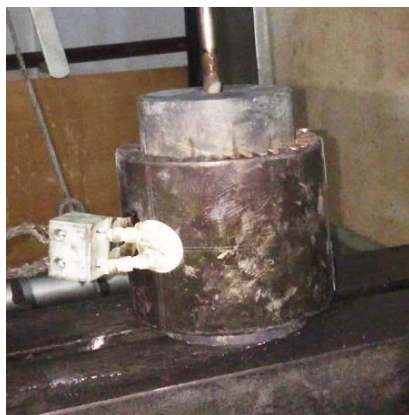
Fig. 3 Schematic illustration of the used extrusion die
