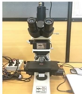
Fig. 5 Used device for measuring Vickers microhardness number
