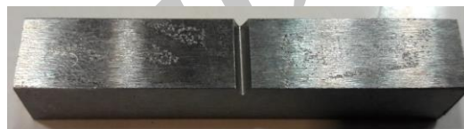
Fig. 8 Impact test sample according to ASTM E 23.
