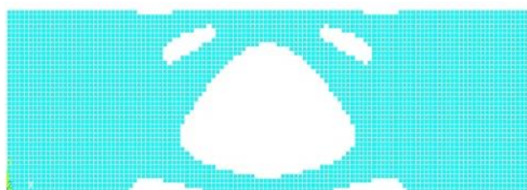
Fig. 8 The final topology of the stiffness-frequency deterministic topology optimization
