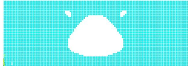
Fig. 9 The final topology of the stiffness-frequency reliability based topology optimization
