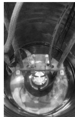
Fig. 4 Electrode system in the water chamber
