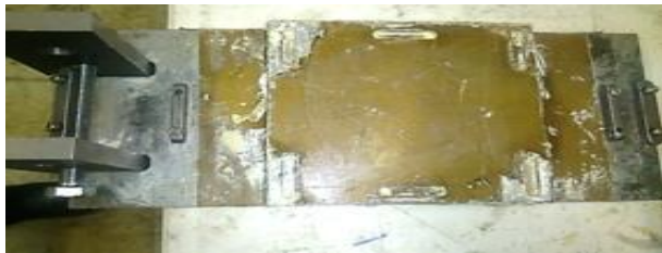
Fig. 2 Mould Manufacturing of fiber metal laminate
